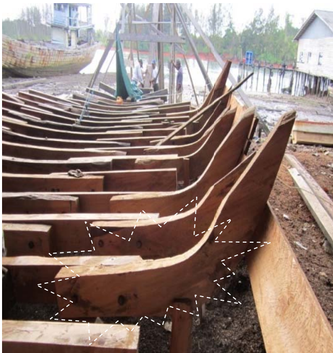
Figure.4: Face knot on the bottom futtock ship.
