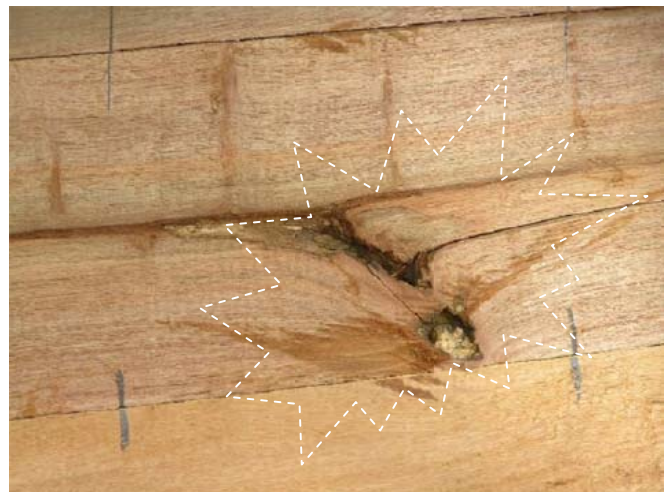
Figure.6: Face knot and shake on the plank ship.
