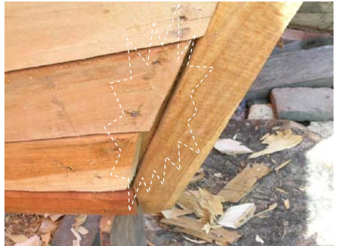
Figure.9: This is one of the most important locations for the attention of all fishermen. because it can cause leaks. The leak is the main enemy for the sailors.
