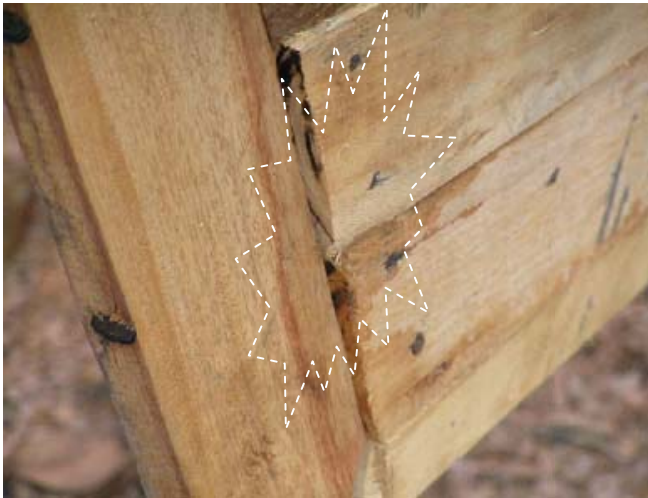
Figure.7: Connections that do not fit part on the forward, would result in the planned thickness of the boards are insatiabile, so that, can be reducing the strength of the vessel until the weakest point,
