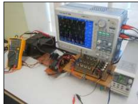
Figure 4: Setup experiment of battery charging from solar PV using DC/DC converter three phase six legs
