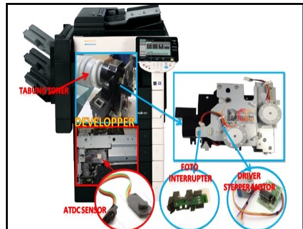
Figure 6: photo interrupter sensor and ATDC sensor
