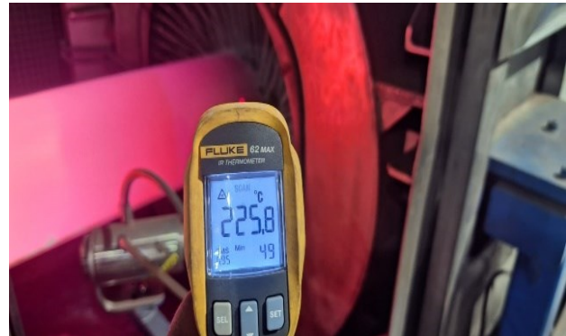
Figure 4a: Temperature inlet quenching chamber
