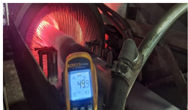
Figure 4b: Temperature outlet quenching chamber
