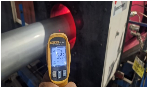
Figure 3a: Temperature inlet coil induction furnace
