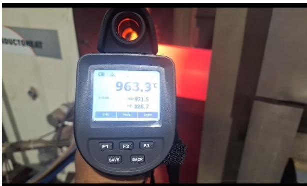
Figure 3b: Temperature outlet coil induction furnace
