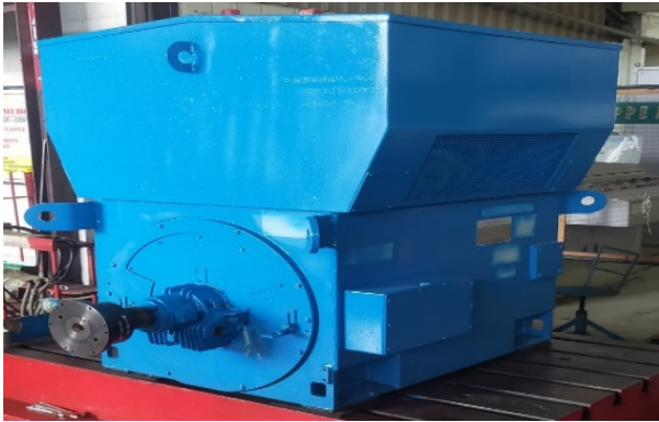
Figure 1: Electric motor 1750 HP
