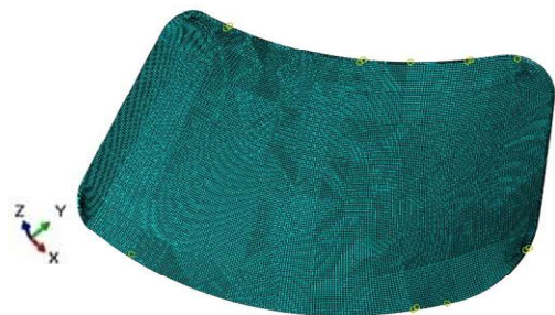
Figure 9: Finite element meshing of the windshield model
