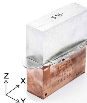
Figure 9: Macroscopic features of joints produced by linear friction welding [53]
